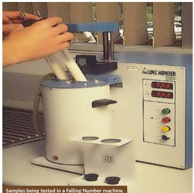
Samples being tested in a Falling Number machine.
